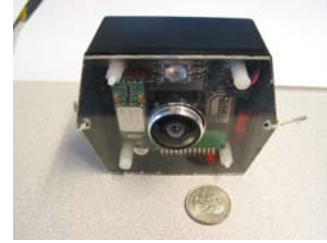
Fig. 2. This smart camera node, which is equipped with an accelerometer, can measure the relative bearing to other sensor nodes or robots.
